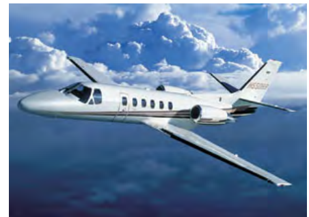
Cessna Citation Bravo (C550) Max. Takeoff Weight: 14,800 pounds Wingspan: 52.17 feet
